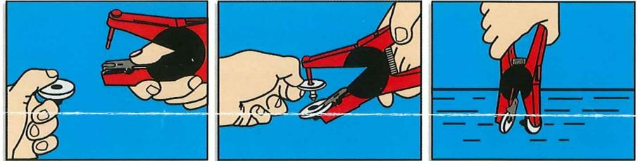
1. To load, depress spring clip and insert the female EID tag. Ensure that the raised portion of the tag, which encloses the transponder chip, is placed in the open portion of the jaws.
